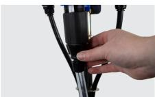
**3.** Screw or Unscrew the adjusting nut so as to bring the top of the nut into ling with relevant injection rate.
