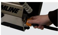
**3.** Connect the Water inlet pipe to the the mains water supply, ensuring you respect all regulations relating to water source
