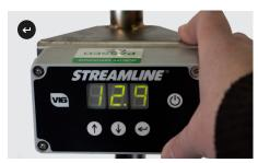
**4.** To switch off the controller, press the power button and hold for 2 seconds.
