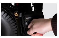
2. Plug charger into mains electrical socket
