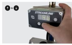
**3.** To check voltage of battery, press the (enter) once, voltage of battery will display. It is recommend any battery lower than 10.8v requires charging.
